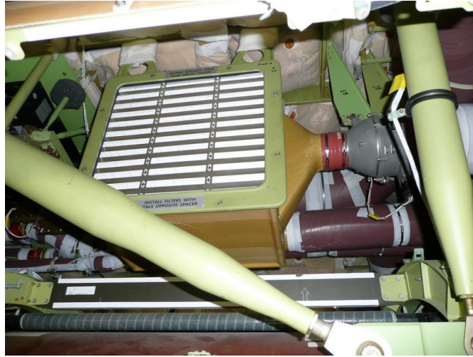
Figure 9: Example of filters in ATA21 (B777)
